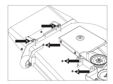
4. Bolt left hand corner mulch baffle to the **outside** of the deck baffle weldment as shown in the illustration.
